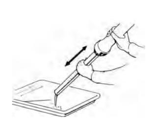
Hold the bottom case in a vice. Remove the socket bolt with an Allen wrench.
