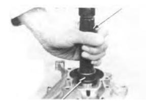
Install the crankshaft bearing into the right crankcase.
