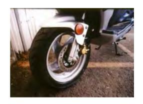
Fill with new brake oil (DOT-3) Release the air in the brake oil passage.
