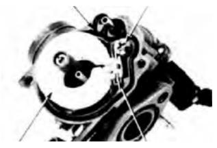
Remove the main jet, slow jet, needle seat & air screw.
