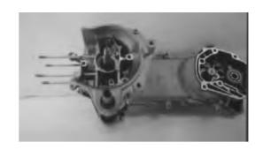
Remove the right crankcase from the left crankcase by using a pulley.
